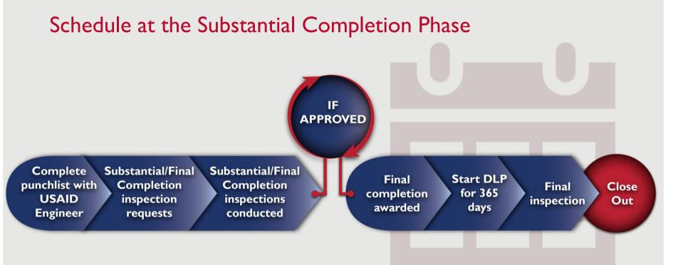
This graphic explains the timeline and process to achieve substantial completion and final closeout. DLP refers to the Defects Liability Period or Warranty period. Schools must be ready for occupancy upon award of Substantial Completion.
